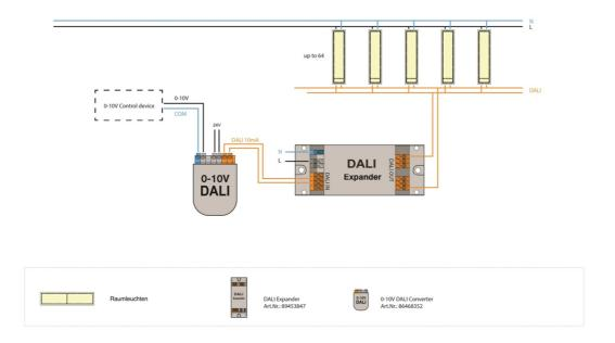
Control of 64 DAL luminares with a 0-10V control device and a 0-10V to DALI converter (ArtNr: 86458352)
