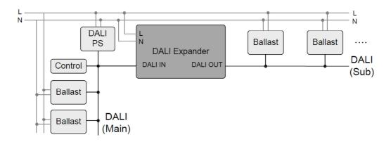
Expansion of a DALI circuit (Main) with a DALI subordinate circuit (all control commands sent to the DALI Expander are sent Broadcast to the DALI sub-circuit.)
