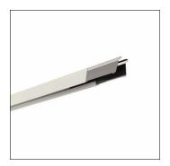
Licross®, trunking rail, of sheet steel, galvanised, coil coated, white, length: 1.500 mm, width: 64 mm, height: 67mm, through-wiring: 9x 2.5mm<sup>2</sup>, protection rating (complete): maximum IP64, depends on used inserts and accessories, insulation class (complete): insulation class I (protective earthing), certification: CE, UKCA, LABS conformity tested according to VDMA 24364:2018-05, packaging unit: 1 piece
