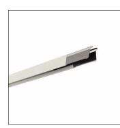
Licross<sup>®</sup>, trunking rail, of sheet steel, galvanised, coil coated, white, length: 3.000 mm, width: 64 mm, height: 67mm, through-wiring: 14x 2.5mm<sup>2</sup>, protection rating (complete): maximum IP64, depends on used inserts and accessories, insulation class (complete): insulation class I (protective earthing), certification: CE, UKCA, LABS conformity tested according to VDMA 24364:2018-05, packaging unit: 1 piece
