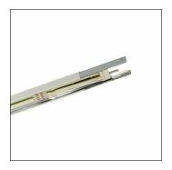
Modario®, trunking rail, of sheet steel, coated, pure white, 2-length, length: 2.392 mm, width: 58 mm, height: 43mm, through-wiring: 10x 2.5mm², with terminal, 10-pole, max. 2.5mm², protection rating (complete): for IP20 protection rating, insulation class (complete): insulation class I (protective earthing), certification: CE, ENEC 10, VDE, standard: EN 60598, packaging unit: 1 piece
