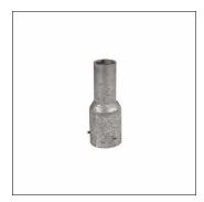
reducer, installation type: post-top, reducing sleeve, of St 37-2, galvanised, length: 350 mm, diameter: 76 mm, spigot size: 89/76mm, packaging unit: 1 piece
