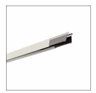
Licross®, trunking rail, of sheet steel, galvanised, coil coated, white, length: 3.000 mm, width: 64 mm, height: 67mm, through-wiring: 9x 2.5mm², protection rating (complete): maximum IP64, depends on used inserts and accessories, insulation class (complete): insulation class I (protective earthing), certification: CE, UKCA, LABS conformity tested according to VDMA 24364:2018-05, packaging unit: 1 piece
