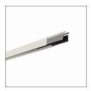
Licross®, trunking rail, of sheet steel, galvanised, coil coated, white, length: 3.000 mm, width: 64 mm, height: 67mm, through-wiring: 11x 2.5mm², protection rating (complete): maximum IP64, depends on used inserts and accessories, insulation class (complete): insulation class I (protective earthing), certification: CE, UKCA, LABS conformity tested according to VDMA 24364:2018-05, packaging unit: 1 piece
