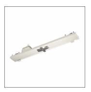
Licross®, rail insert, adapter,with plug, 5-pole, with phase selection, mains connection: 230V, AC, 50/60Hz, terminal,5-pole, max. 2.5mm², multi adapter, of sheet steel, coil coated, white, for IP20/IP40 protection rating, length: 500mm, width: 64mm, height: 68mm, multifunctional insert, protection rating (complete): IP20, insulation class (complete): insulation class I (protective earthing), certification: CE, UKCA, packaging unit: 1 piece
