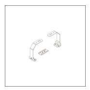
Highbay 11, ceiling mounting, installation type: surface-mounted, ceiling mounting bracket, of steel, galvanised, length: 165mm, width: 40mm, height: 150mm, packaging unit: set of 2
