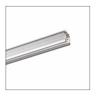
AX T, 3-phase track, installation type: suspended mounting, surface-mounted, mains connection: 220..240V/380..400V, AC, of extruded aluminium section, coated, grey, length: 2.000 mm, width: 32 mm, height: 33mm, protection rating (complete): IP20, insulation class (complete): insulation class I (protective earthing), certification: CE, ENEC, packaging unit: 1 piece
