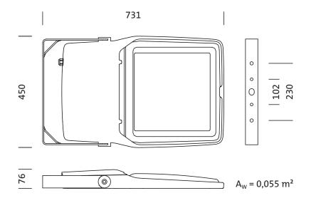
It is mandatory that the assembly instructions must be observed when planning and installing the electrical installation (to be found at www.siteco.de) Tolerances related to thermal, electrical and photometric data according to IEC 62722 Issued 13.04.2024 - Modifications and errors subject to change - Ensure that you always use the latest version -
