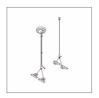
Apollon<sup>®</sup> 2, Y-wire suspension, ceiling sleeve, with with 2 terminals, 1-pole, max. 2.5mm<sup>2</sup>, connection cable,2X0.75mm<sup>2</sup>, ceiling fixing element, of steel, galvanised, ceiling canopy, of plastic, wire, of steel, galvanised, fixing on luminaire side, of steel, galvanised, ceiling sleeve, of steel, nickel-plated, packaging unit: set of 2
