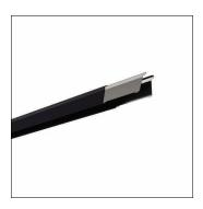
Licross®, trunking rail, of sheet steel, galvanised, coil coated, matt jet black (RAL 9005), length: 1.500 mm, width: 64 mm, height: 67mm, through-wiring: 11x 2.5mm², protection rating (complete): maximum IP64, depends on used inserts and accessories, insulation class (complete): insulation class I (protective earthing), certification: CE, UKCA, LABS conformity tested according to VDMA 24364:2018-05, packaging unit: 1 piece
