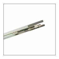
Modario®, trunking rail, of sheet steel, coated, pure white, 2-length, length: 2.392 mm, width: 58 mm, height: 43mm, through-wiring: 5x 2.5mm², with terminal, 5-pole, max. 2.5mm², protection rating (complete): for IP20 protection rating, insulation class (complete): insulation class I (protective earthing), certification: CE, ENEC 10, VDE, standard: EN 60598, packaging unit: 1 piece
