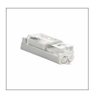
cable junction box, for 3 cables to 5x 10mm<sup>2</sup>, L1/L2/L3/N/PE(N), 2x E14, cable junction box, of plastic, shock-resistant, inner mast diameter: from 84mm, protection rating (complete): IP44, insulation class (complete): insulation class II (safety insulation), certification: CE, packaging unit: 1 piece
