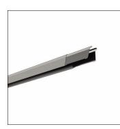
Licross<sup>®</sup>, trunking rail, of sheet steel, galvanised, coil coated, metallic grey (RAL 9006), length: 3.000 mm, width: 64 mm, height: 67mm, through-wiring: 14x 2.5mm<sup>2</sup>, protection rating (complete): maximum IP64, depends on used inserts and accessories, insulation class (complete): insulation class I (protective earthing), certification: CE, UKCA, LABS conformity tested according to VDMA 24364:2018-05, packaging unit: 1 piece
