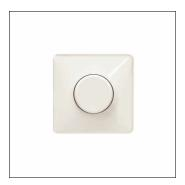
SITECO Connect 41 Rotaryrotary dimmer, Touchdim, local control, dimmable, installation type: recessed, installation location: in the switch box, of plastic, protection rating (complete): IP20, insulation class (complete): insulation class II (safety insulation), certification: CE, voltage: 230V, voltage type: AC, 1 x rotary button/push button, 1 x DALI, packaging unit: 1 piece
