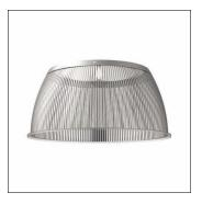
Highbay 31 S, reflector, primary light control with reflector, of PC, transparent prismatic structure, light emission: direct with ceiling illumination distribution, primary light characteristic: rotationally symmetric, installation type: surface-mounted, diameter: 480mm, height: 227mm, packaging unit: 1 piece
