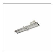
Licross® Trunkingsensor module PC3-S, slave, central control, dimmable, installation location: to the Licross® trunking rail, of sheet steel, protection rating (complete): IP20, insulation class (complete): insulation class I (protective earthing), certification: CE, UKCA, 1 x PIR movement sensor, 1 x light sensor, packaging unit: 1 piece
