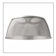
Highbay 31 L, reflector, primary light control with reflector, of PC, transparent prismatic structure, light emission: direct with ceiling illumination distribution, primary light characteristic: rotationally symmetric, installation type: surface-mounted, diameter: 570mm, height: 234mm, packaging unit: 1 piece
