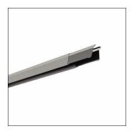
Licross®, trunking rail, of sheet steel, galvanised, coil coated, metallic grey (RAL 9006), length: 4.500 mm, width: 64 mm, height: 67mm, through-wiring: 7x 2.5mm², protection rating (complete): maximum IP64, depends on used inserts and accessories, insulation class (complete): insulation class I (protective earthing), certification: CE, UKCA, LABS conformity tested according to VDMA 24364:2018-05, packaging unit: 1 piece
