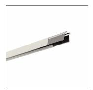
Licross®, trunking rail, of sheet steel, galvanised, coil coated, white, length: 4.500 mm, width: 64 mm, height: 67mm, through-wiring: 7x 2.5mm², protection rating (complete): maximum IP64, depends on used inserts and accessories, insulation class (complete): insulation class I (protective earthing), certification: CE, UKCA, LABS conformity tested according to VDMA 24364:2018-05, packaging unit: 1 piece
