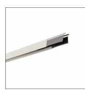
Licross<sup>®</sup>, trunking rail, of sheet steel, galvanised, coil coated, white, length: 3.000 mm, width: 64 mm, height: 67mm, through-wiring: 7x 2.5mm<sup>2</sup>, protection rating (complete): maximum IP64, depends on used inserts and accessories, insulation class (complete): insulation class I (protective earthing), certification: CE, UKCA, LABS conformity tested according to VDMA 24364:2018-05, packaging unit: 1 piece
