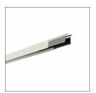
Licross®, trunking rail, of sheet steel, galvanised, coil coated, white, length: 4.500 mm, width: 64 mm, height: 67mm, protection rating (complete): maximum IP64, depends on used inserts and accessories, insulation class (complete): insulation class I (protective earthing), certification: CE, UKCA, LABS conformity tested according to VDMA 24364:2018-05, packaging unit: 1 piece
