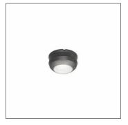
SITECO Connect WirelessMotion Low, Smart Interface below, setting of the ECG to logarithmic DALI dimming required, installation type: screw fastening, installation location: to the luminaire, of plastic, voltage: 24V, voltage type: DC, Bluetooth, D4i, local setting and operation with smartphone app, by daylight, by movement, 1 PIR movement sensor, daylight sensor, PIR movement sensor, protection rating (complete): IP66, certification: CE, UKCA, packaging unit: 1 piece
