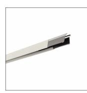
Licross<sup>®</sup>, trunking rail, of sheet steel, galvanised, coil coated, white, length: 4.500 mm, width: 64 mm, height: 67mm, through-wiring: 14x 2.5mm<sup>2</sup>, protection rating (complete): maximum IP64, depends on used inserts and accessories, insulation class (complete): insulation class I (protective earthing), certification: CE, UKCA, LABS conformity tested according to VDMA 24364:2018-05, packaging unit: 1 piece
