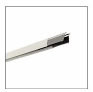
Licross®, trunking rail, of sheet steel, galvanised, coil coated, white, length: 1.500 mm, width: 64 mm, height: 67mm, through-wiring: 14x 2.5mm², protection rating (complete): maximum IP64, depends on used inserts and accessories, insulation class (complete): insulation class I (protective earthing), certification: CE, UKCA, LABS conformity tested according to VDMA 24364:2018-05, packaging unit: 1 piece
