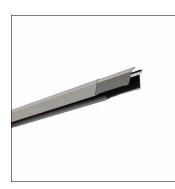
Licross<sup>®</sup>, trunking rail, of sheet steel, galvanised, coil coated, metallic grey (RAL 9006), length: 4.500 mm, width: 64 mm, height: 67mm, protection rating (complete): maximum IP64, depends on used inserts and accessories, insulation class (complete): insulation class I (protective earthing), certification: CE, UKCA, LABS conformity tested according to VDMA 24364:2018-05, packaging unit: 1 piece
