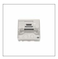
SITECO ConnectExternal Interface MD, master, local control, dimmable, installation type: surface-mounted, installation location: to the ceiling, to the luminaire, of plastic, protection rating (complete): IP54, insulation class (complete): insulation class II (safety insulation), certification: CE, VDE, voltage: 230V, voltage type: AC, packaging unit: 1 piece
