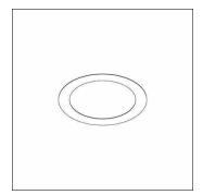
Lunis 21, adapter, installation type: surface-mounted, adapter, of aluminium, traffic white (RAL 9016), diameter: 200mm, packaging unit: set of 5
