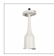
electrics components group, for Module 540 iQ, gear tray, control gear: ECG iQ, LED luminous flux: 1.610 lm, colour temperature: 3000K, with terminal, 6-pole, max. 2.5mm<sup>2</sup>, mains connection: 230..240V, AC, 50/60Hz, start of lifetime: 11 W, end of service life: 11 W, reduction: 5 W, primary light characteristic: asymmetric, width: 190 mm, height: 514mm, insulation class (complete): insulation class II (safety insulation), certification: CE, ENEC, VDE
