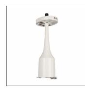
electrics components group, for Module 540 iQ, gear tray, control gear: ECG iQ, LED luminous flux: 1.590 lm, colour temperature: 2700K, with terminal, 6-pole, max. 2.5mm<sup>2</sup>, mains connection: 230..240V, AC, 50/60Hz, start of lifetime: 12 W, end of service life: 12 W, reduction: 6 W, primary light characteristic: strongly asymmetric, width: 190 mm, height: 514mm, insulation class (complete): insulation class II (safety insulation), certification: CE, ENEC, VDE
