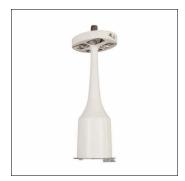
electrics components group, for Module 540 iQ, gear tray, control gear: ECG iQ, LED luminous flux: 5.150 lm, colour temperature: 4000K, with terminal, 6-pole, max. 2.5mm², mains connection: 230..240V, AC, 50/60Hz, start of lifetime: 34 W, end of service life: 36 W, reduction: 15 W, primary light characteristic: strongly asymmetric, width: 190 mm, height: 514mm, insulation class (complete): insulation class II (safety insulation), certification: CE, ENEC, VDE
