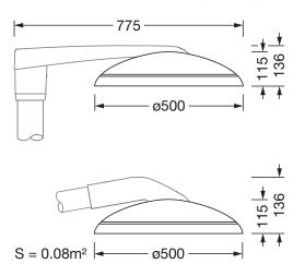
It is mandatory that the assembly instructions must be observed when planning and installing the electrical installation (to be found at www.siteco.de) Tolerances related to thermal, electrical and photometric data according to IEC 62722 Issued 16.02.2024 - Modifications and errors subject to change - Ensure that you always use the latest version -
