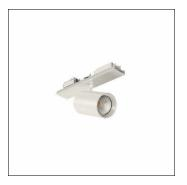
Licross® Spot 31, directional spotlight, light control with lens, of plastic, LED rated luminous flux: 5.140lm, light colour: 940, with plug, 3-pole, with phase selection, mains connection: 220..240V, AC, 50/60Hz, of aluminium, traffic white (RAL 9016), length: 300mm, diameter: 90mm, protection rating (complete): IP20, insulation class (complete): insulation class I (protective earthing), certification: CE, packaging unit: 1 piece
