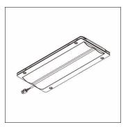
Streetlight 10 mini/midi, LED module, primary light control with cycle path optic, light distribution: P1.0a, primary light characteristic: asymmetric, High Power LED, light colour: 722, colour temperature: 2200K, mains connection: 230..240V, 50Hz, LED module, length: 310mm, width: 137mm, height: 40mm, protection rating (complete): as luminaire, packaging unit: 1 piece
