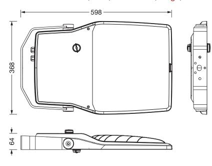
It is mandatory that the assembly instructions must be observed when planning and installing the electrical installation (to be found at www.siteco.de) Tolerances related to thermal, electrical and photometric data according to IEC 62722 Issued 23.05.2025 - Modifications and errors subject to change - Ensure that you always use the latest version -
